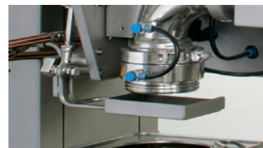
90° curved valve with drip catcher
