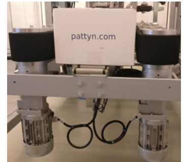
Robust side belts, driven by 2 motors
