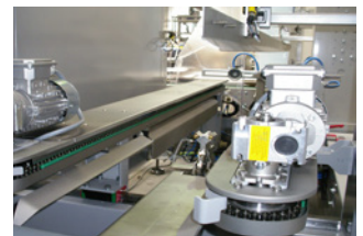
Synchronised chain system
