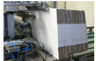
Failsafe carton separator
